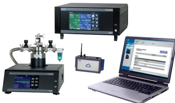
**Modello CPU6000-W, CPC6050, CPD8500 e PC con software WIKA-Cal**
