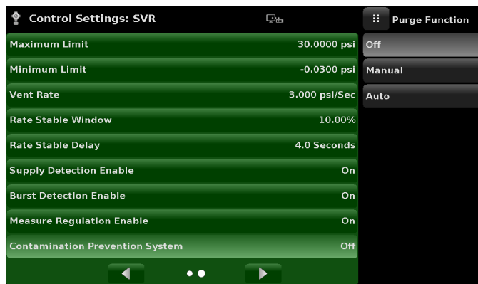
Fig. 8.9.2.3-B - Contamination prevention system
