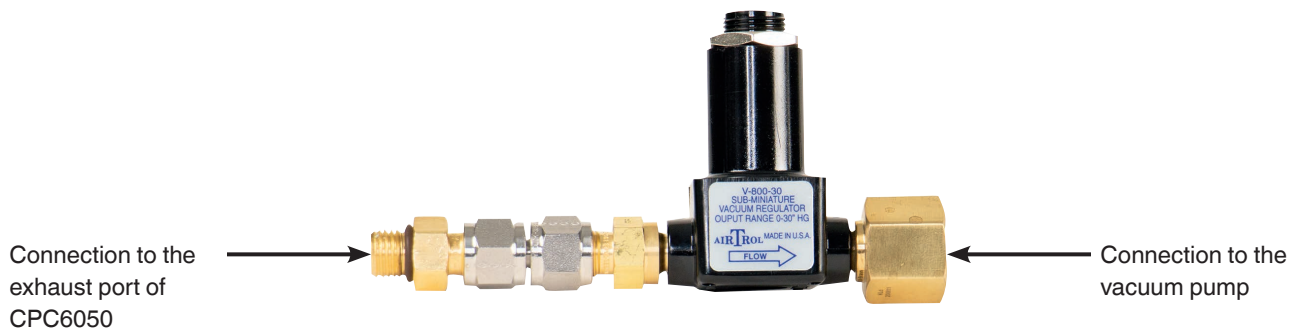
Fig. 8.11-B - Vacuum regulator
