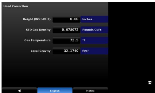
Figure 7-45 Head Correction Screen english units
