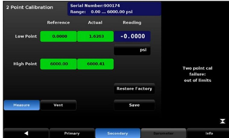
Figure 6.4.2.5.2-9 – ‘2 Point Calibration Failure’]
