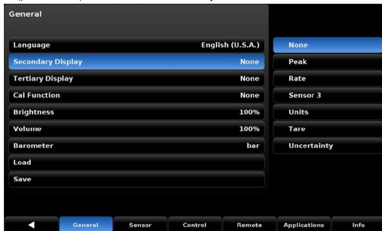
Figure 6.4.2.1.2 Auxiliary Displays
