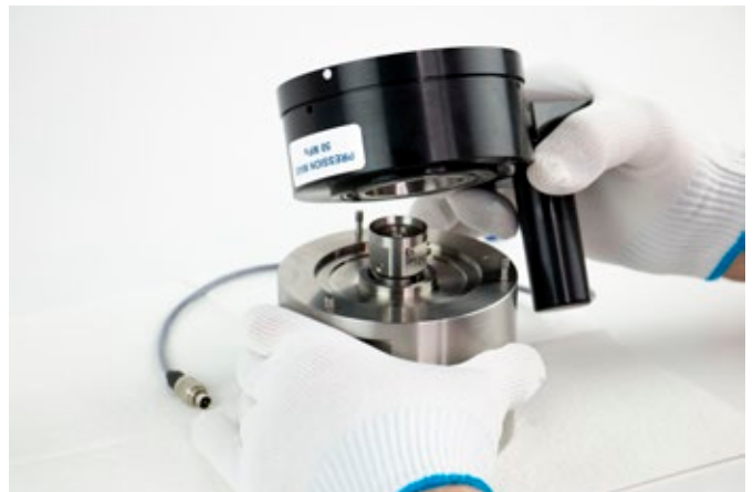
Figure 8.1.2.3.1-A Separating Measuring Head
