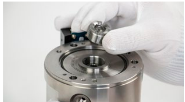
Figure 8.1.2.2.1-E Removing the cylinder jam nut
