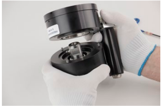
Figure 8.1.2.2.1-A Separating Measuring Head
