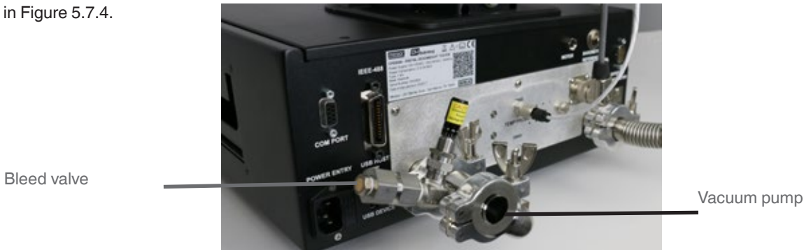
Figure 5.7.4 CPD8500 Absolute Rear Panel Connections
