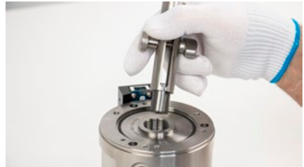
Figure 8.1.2.2.1-F Removing the cylinder
