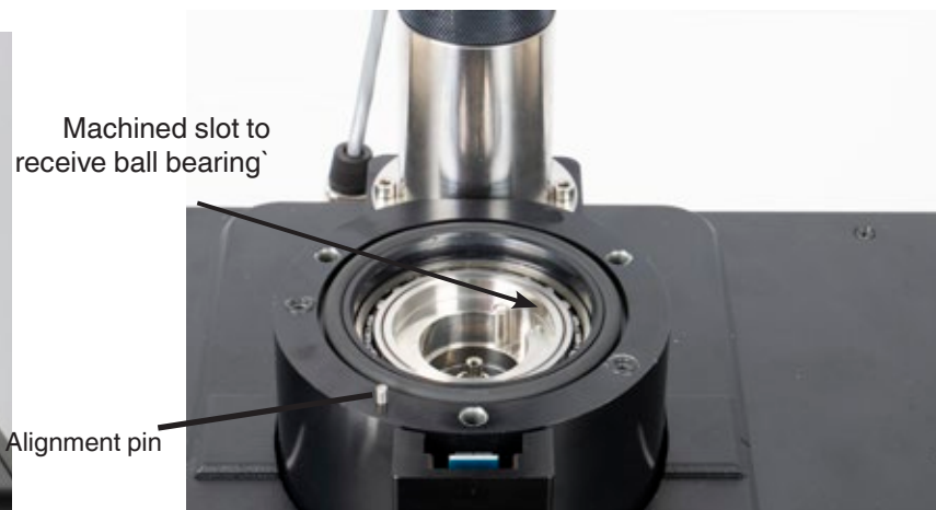
Figure 5.4.1-F Machined slot in Base
