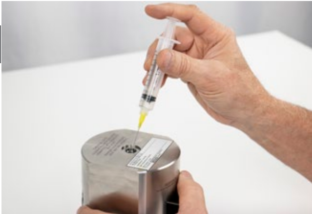
Figure 5.4.2-F Adding Oil to the Gauge Head
