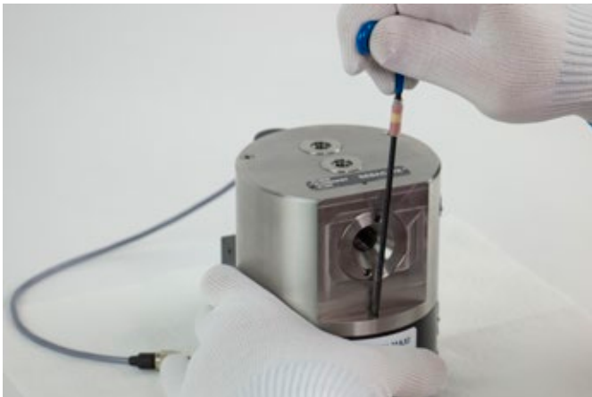
Figure 8.1.2.3.1-A Separating Measuring Head
