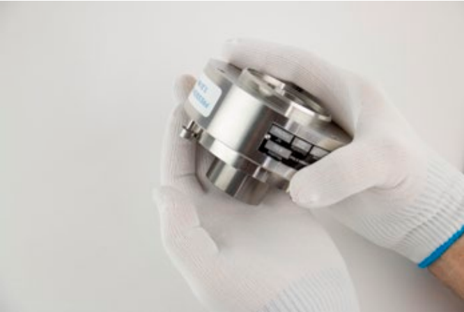
Figure 8.1.2.1.1-D Removing Cylinder From Head
