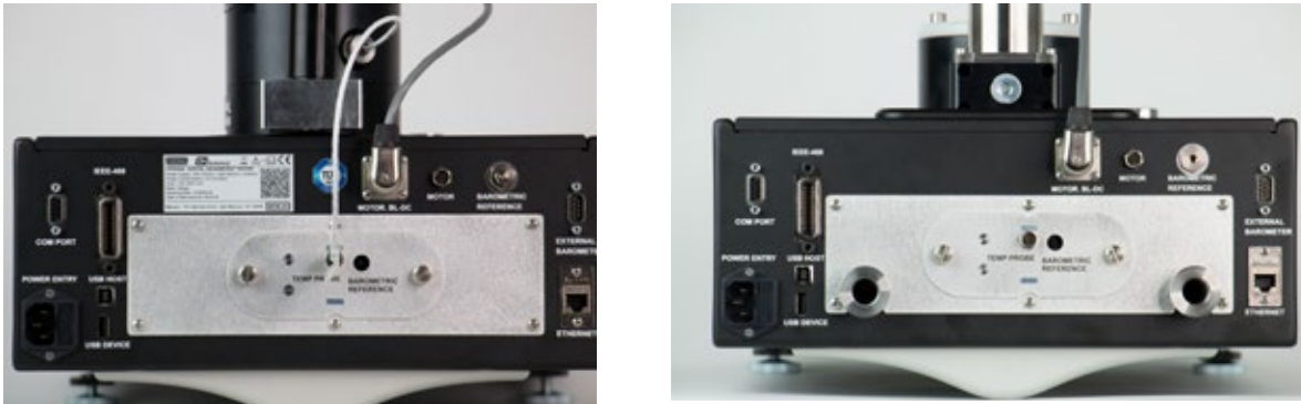
Figure 5.10-A Rear Panel - Gauge (left) and Absolute (right)
