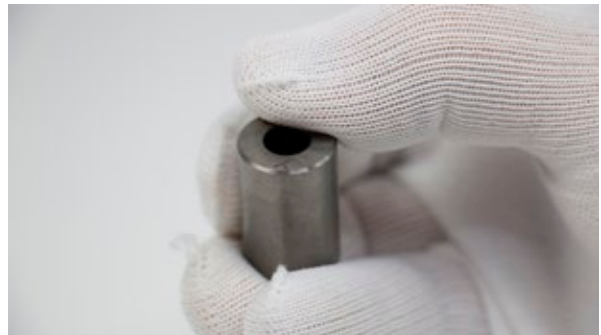
Figure 8.1.2.2.2-B Cylinder with chamfer and markings for insertion
