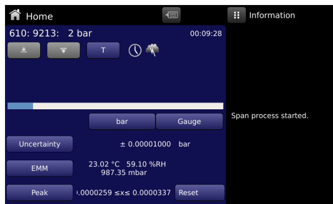
Figure 6.4.1.4-C Span Calibration Process
