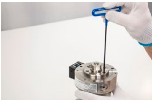
Figure 8.1.2.1.1-A Removing retaining ring
