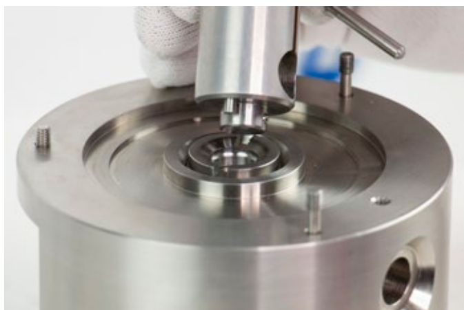
Figure 8.1.2.3.1-C Jam Nut Removal
