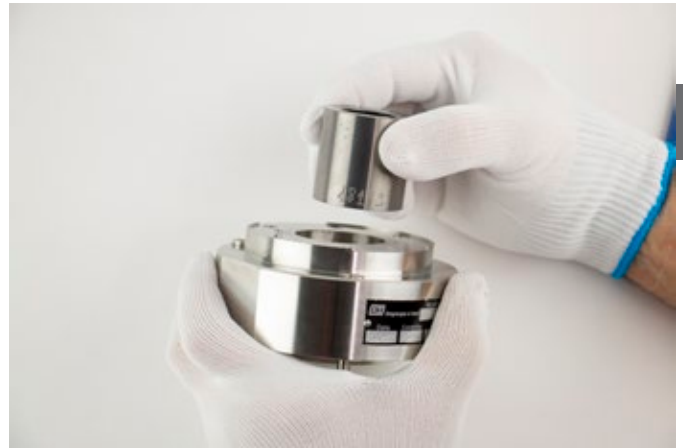
Figure 8.1.2.1.1-D Removing Cylinder From Head
