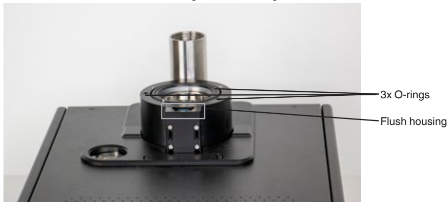
Fig 5.8.1-D Check O-rings and housing
