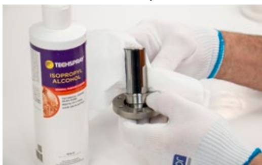
Figure 8.1.2.1.2-A Piston and cylinder cleaning
