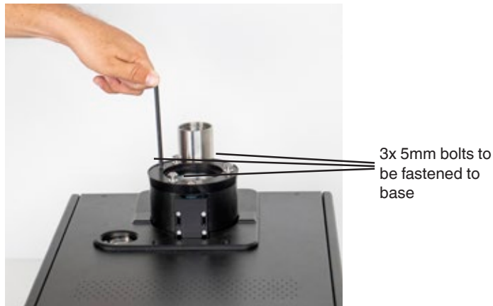
Fig 5.8.2-B Install gauge adapter
