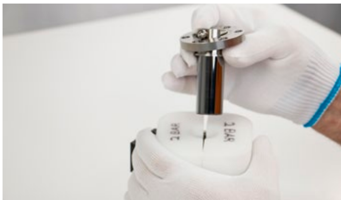
Figure 8.1.2.1.1-C Removing the piston
