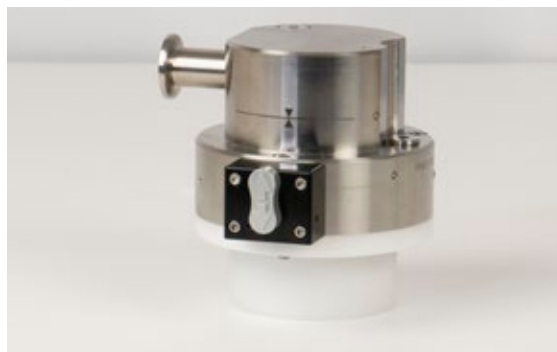
Figure 8.1.2.1-A CPS8500A measuring head
