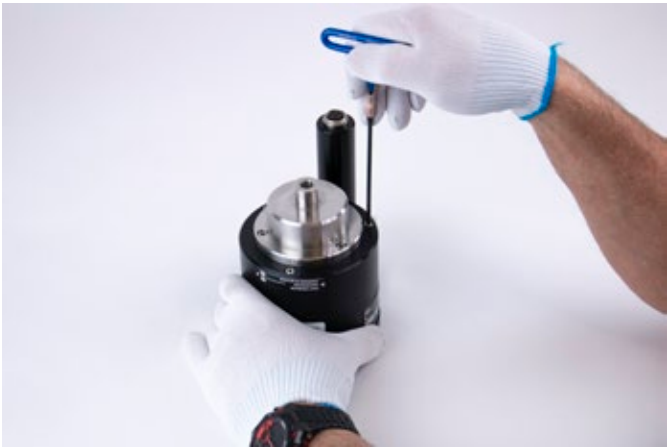
Figure 8.1.2.2.1-A Separating Measuring Head
