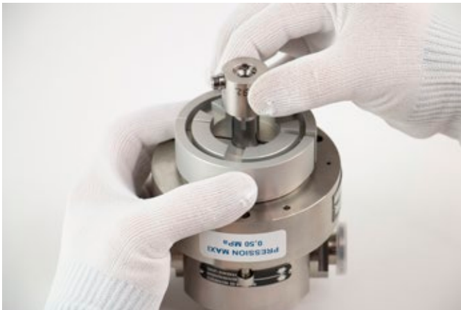
Figure 8.1.2.1.3 Measuring Head Reassembly
