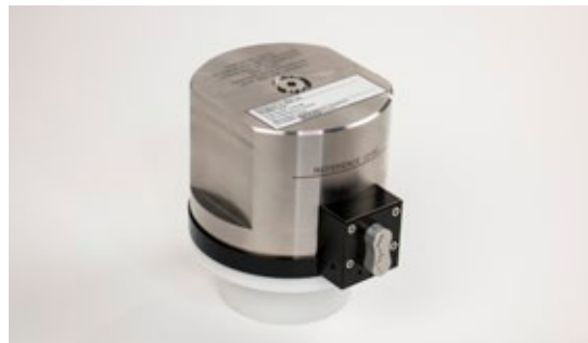
Figure 8.1.2.2-A CPS8500G Measuring Head
