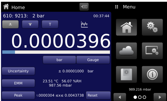
Figure 6.4.1.1-B Unstable Pressure Reading
