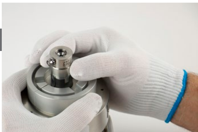
Figure 8.1.2.1.1-A Removing The Piston From Head
