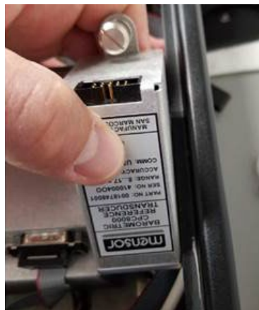
Figure 8.1.3.5-B Barometric Reference Removal
