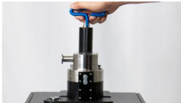
Figure 5.4.1-H Fastening CPS8500A to the base
