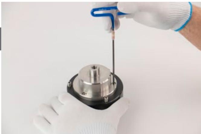
Figure 8.1.2.2.1-C Cylinder With Top Cap
