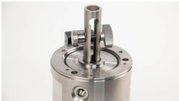
Figure 8.1.2.2.1-F Removing the cylinder
