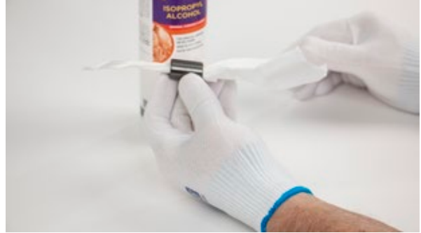
Figure 8.1.2.2.2-A Cleaning the piston and cylinder
