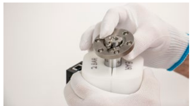
Figure 8.1.2.1.1-B Piston removal tool
