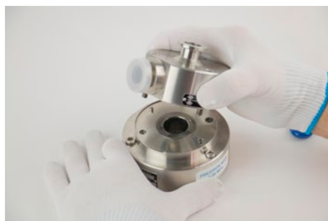
Figure 8.1.2.1.1-B Removing Top Cap
