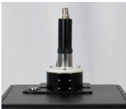
Figure 5.4.1-E Protective cap on Base
