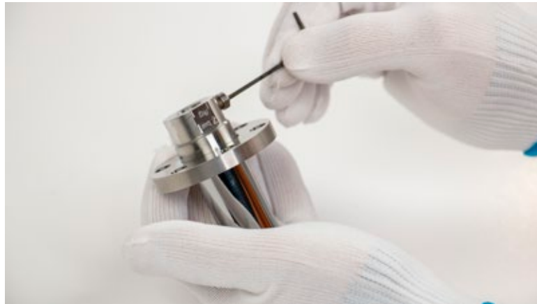
Figure 8.1.2.1.2-B Removing piston retaining ring
