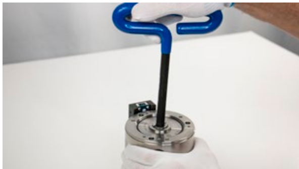
Figure 8.1.2.2.1-E Removing the cylinder jam nut
