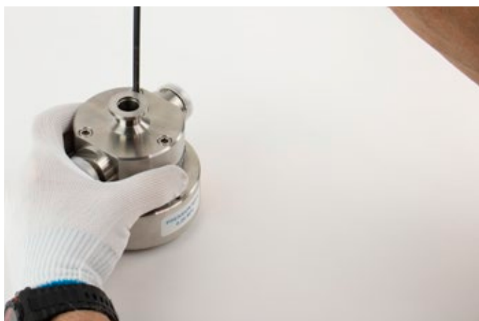
Figure 8.1.2.1.1-B Removing Top Cap
