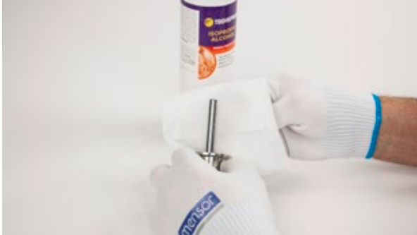
Figure 8.1.2.2.2-A Cleaning the piston and cylinder
