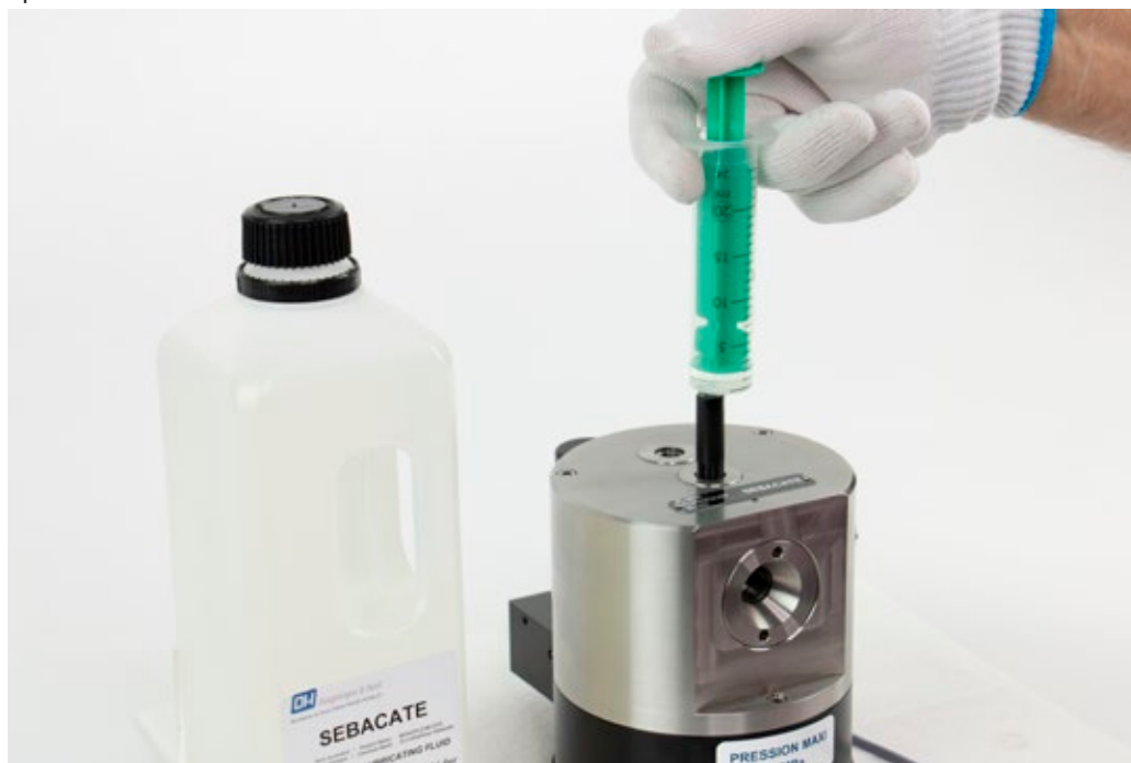
Figure 8.1.2.3.3-A Oil Filling Process
