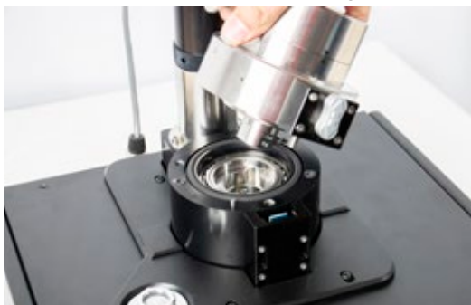
Figure 5.4.1-G Aligning the CPS8500A
