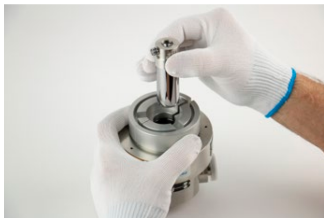
Figure 8.1.2.1.1-A Removing The Piston From Head
