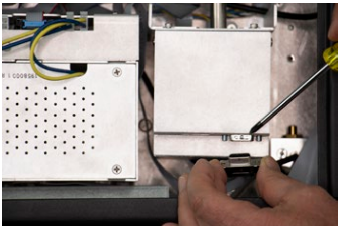
Figure 8.1.3.4-C Unplugging Vacuum Transducer
