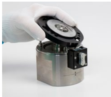
Figure 8.1.2.2.1-B Removing Bayonet Ring
